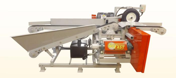
The 6 x 6 Master Return Resaw is very similar to our 6 x 8 Master Resaws. This automatic return resaw is equipped with a powered hold-down and an innovative powered belt return, which is self adjusting and offers operators the ability to fine-tune the return belt height and angle to fit your specific mix of products. When setting the sawblade to the desired board thickness, the feed belt conveyor and the return belt are all simultaneously adjusted to maintain optimum height for peak performance
